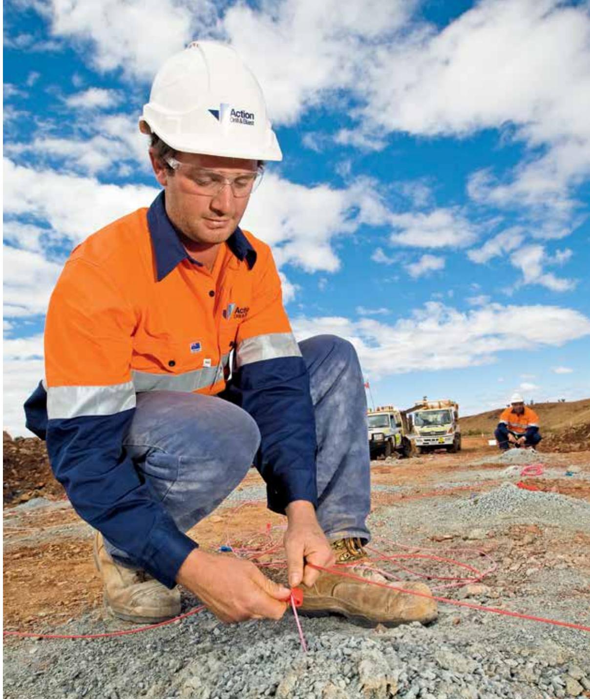
A shotfirer tying in a blast hole.
